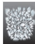
Breakage of Full Surface Physical Toughened glassware
